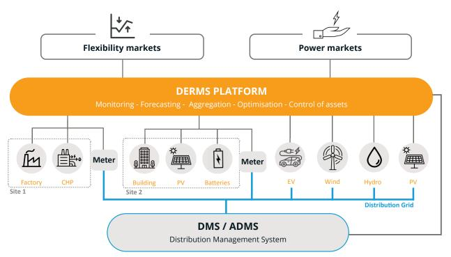
In this configuration, the DERMS provides you with a full access to "Behind the meter" and "grid connected" assets, and to market platforms, as well as advanced forecasting, optimisation and control features.
