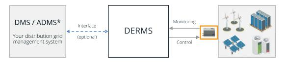
In this configuration, Energy Pool's DERMS gives you access to the distributed energy resources, whether they are directly connected to the grid, or "behind the meter". Data can be exchanged with your DMS/ADMS through an interface.
